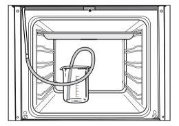
4 Place the container with the descaling solution on the floor of the oven.
